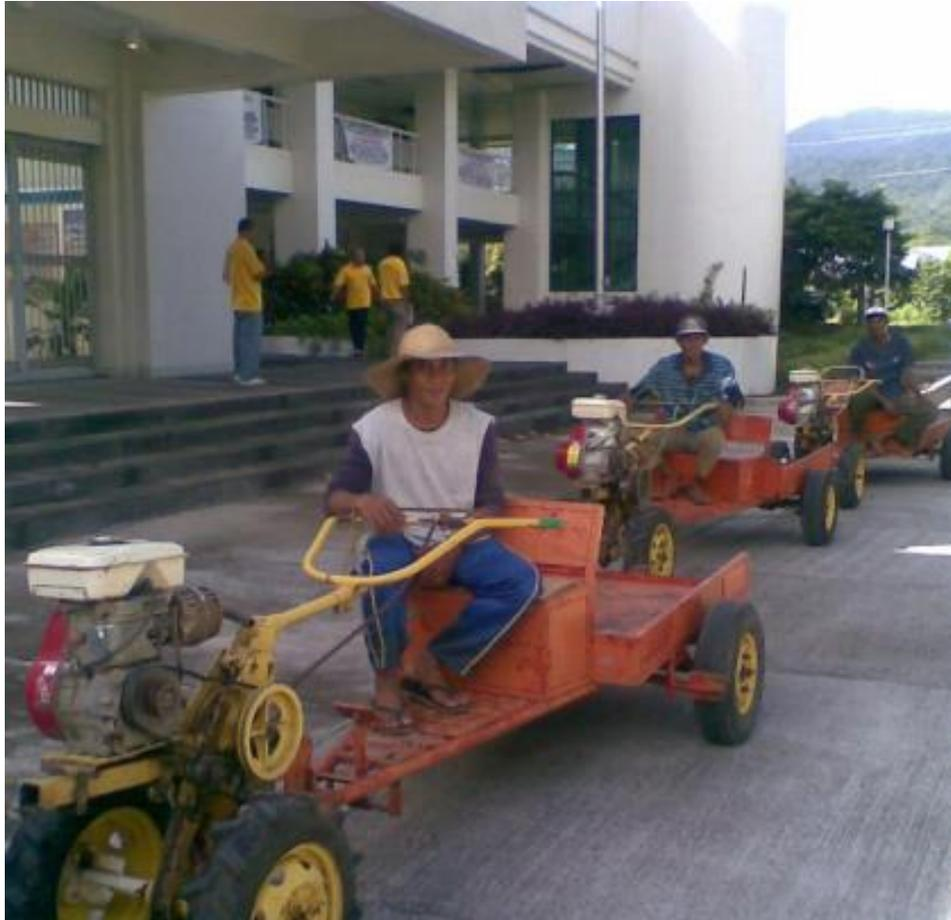
The power-tiller itself can be used to move equipment fitted to the tractor hitch. Additional rubber tyres can be used for transport. All tiller attachments are accommodated in the trailer including cage wheel, plough harrow and counterweight.
