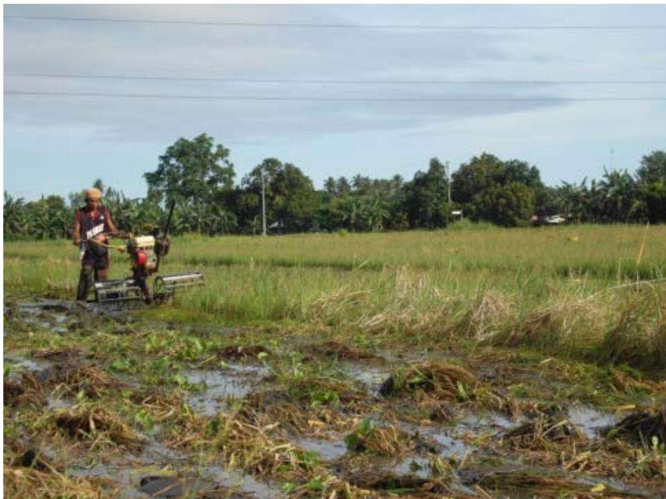
The power-tiller ploughs, puddles, cultivates and transports. Tiller mounted with 6 hp air-cooled gasoline engine with moldboard plough attachment and steel cage wheel for ploughing operation. Average field capacity of 0.6 ha/day.
