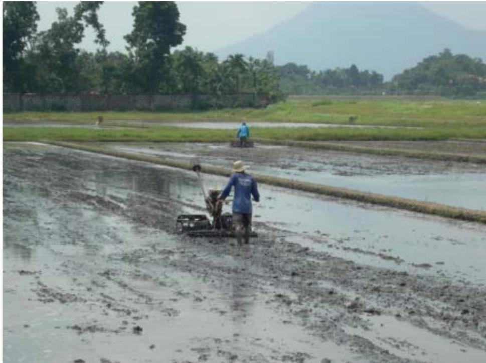
A power-tiller mounted with a 6 hp air-cooled gasoline engine with comb harrow attachment and steel cage wheel for harrowing. Average field capacity of 1.5 ha/day for final harrowing.
