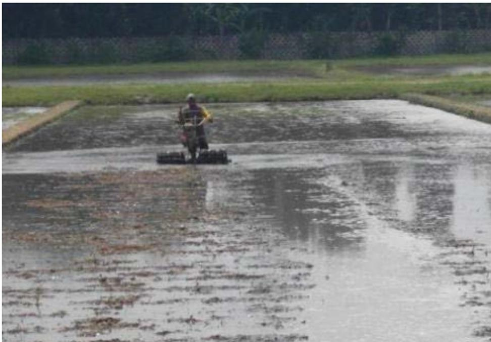
A power-tiller mounted with a 6 hp air-cooled gasoline engine with comb harrow attachment and steel cage wheel for harrowing. Average field capacity of 1.25 ha/day.
