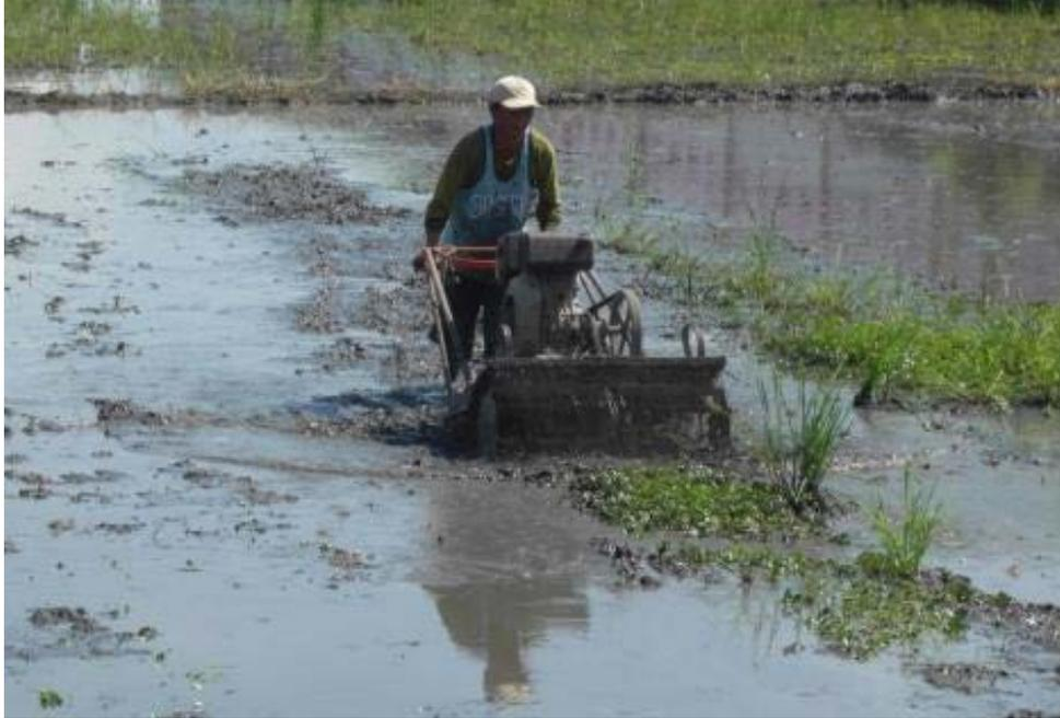
A 1-m swath hydro-tiller/float-tiller mounted with 10 hp air-cooled diesel engine operates both on standard and extreme field conditions having deep mud and/or water. Average puddling field capacity of 1.25 ha/day depending on soil conditions.
