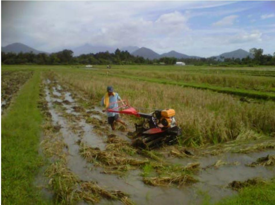
The power-tiller ploughs, puddles, cultivates and transports. Tiller mounted with 7 hp air-cooled gasoline engine with moldboard plough attachment and steel cage wheel for ploughing. Average field capacity of 1 ha/day at machine speed of 3.5 km/h.
