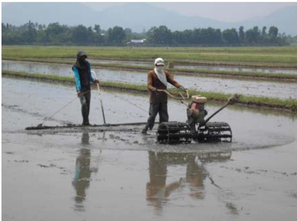
A power-tiller mounted with a 6 hp air-cooled gasoline engine with steel cage wheel attachment for final levelling of paddy field. A 3-m long levelling board with handle is used. Average field capacity of 1.5 ha/day
